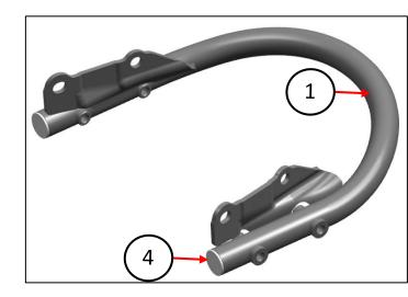
**4.** Assemble Rear Rail Assembly (1) on sub frame by Using Four M8x16 screw (2) & washer (3).
