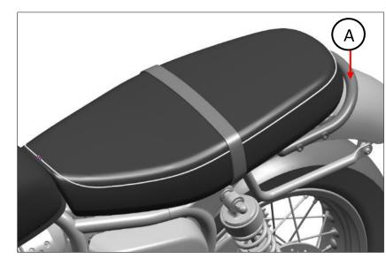
**1.** Assemble grab rail assembly (1) on Rear rail by using four M8x16 screw (2)
