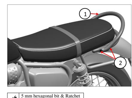
Tighten the bolt to 25 Nm
